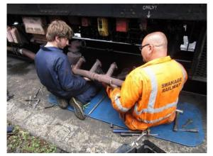
Adam and Andy finally have the awkwardly located exhaust manifold off the engine.
