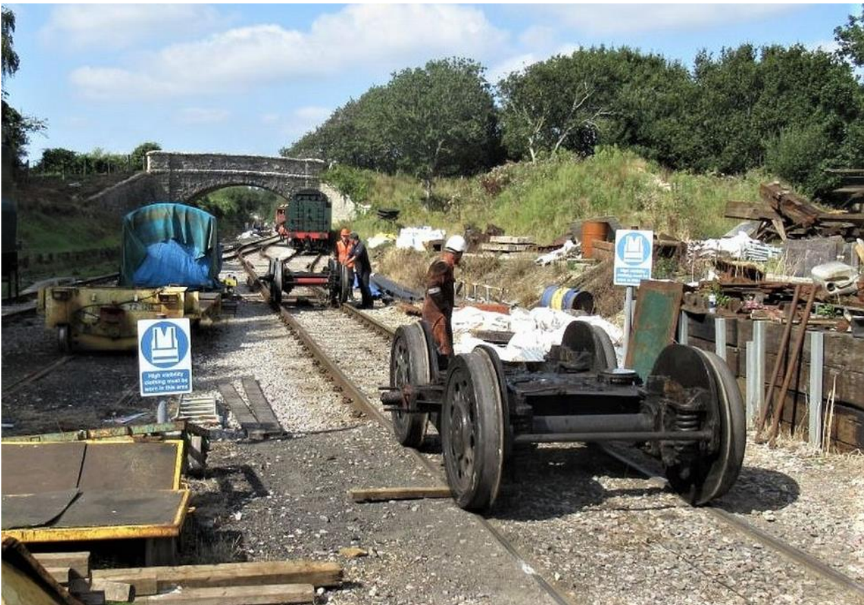
Eddystone has been parted from its tender and the front end lifted to release the bogie. Steam Superintendent Graham Froud , fitter Chris Birmingham and Southern Locos fitter Bailey England manually push the bogie to the other end of the Arne Road siding and push the bogie from 3407 Wadebridge back underneath.
