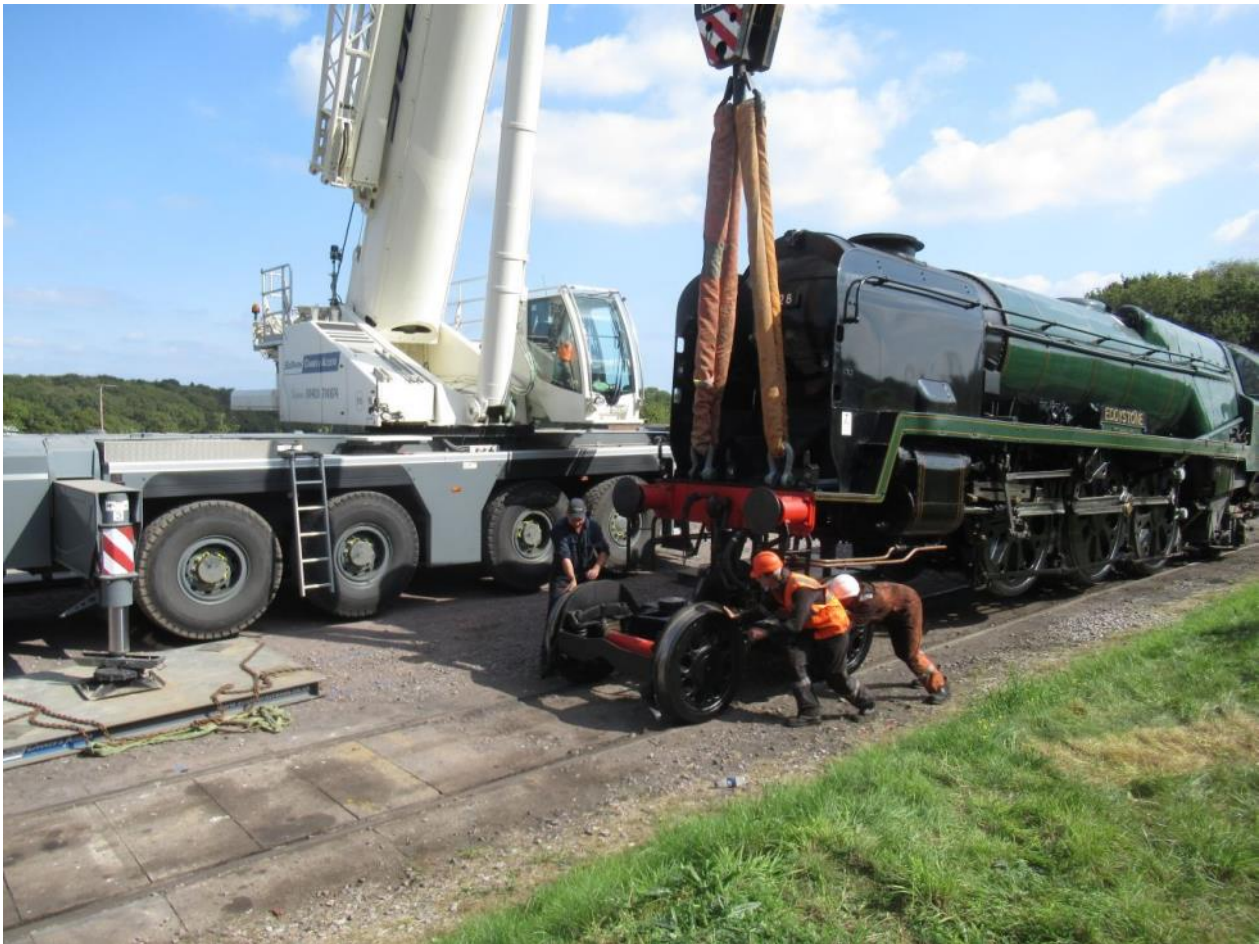
Eddystone has been parted from its tender and the front end lifted to release the bogie. Steam Superintendent Graham Froud , fitter Chris Birmingham and Southern Locos fitter Bailey England manually push the bogie to the other end of the Arne Road siding and push the bogie from 3407 Wadebridge back underneath.
