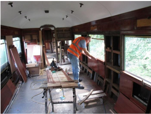
Further down the coach, Mark Humphries does a trial fit of a new side panel,
