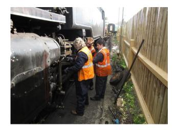
In order to fit new cylinder liners, the cylinders are bored out with a boring bar fixed to the cylinder ends.
