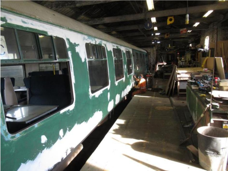
Inside the shed, Tourist Second Open (TSO) no. S4945 is undergoing overhaul, with fitter Jason Kingdon engaged in body repairs. All that filler makes it look worse than it really is.
