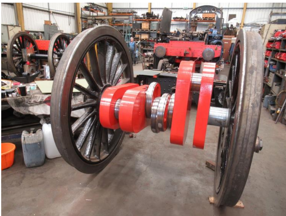
The leading driving axle, with bearing journals and valve eccentrics all nice and shiny!
