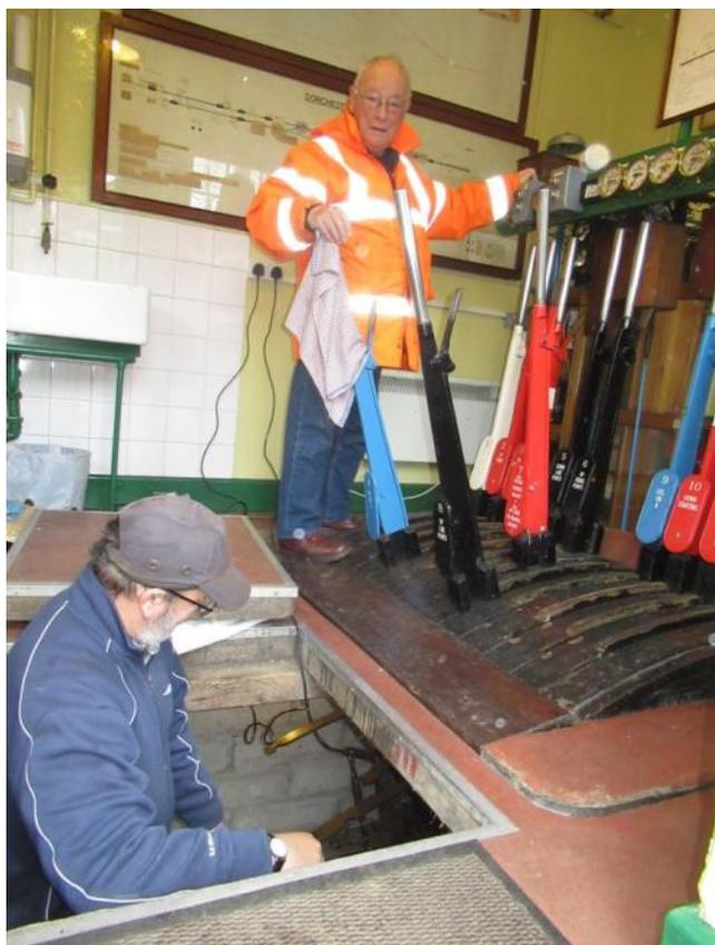
Marco is in the pit underneath the frame making adjustments, while Tony pulls the levers and checks the instruments.
