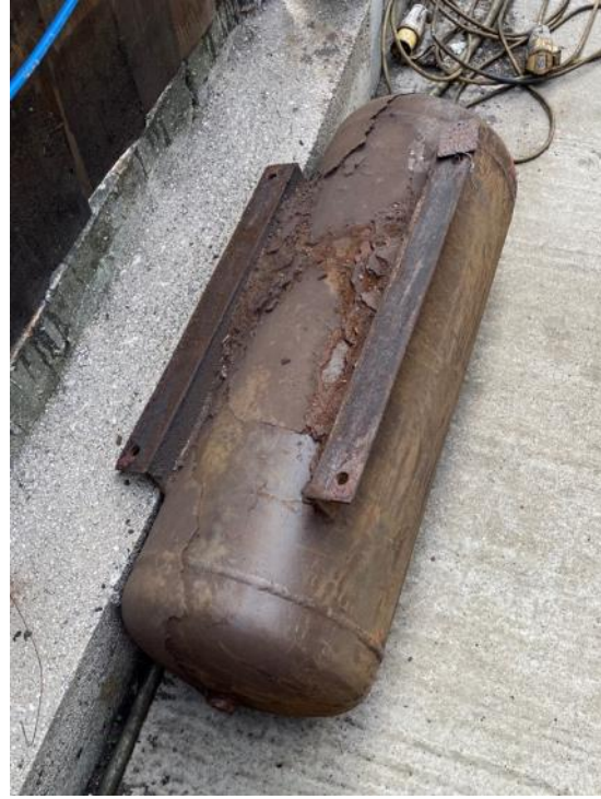
Old air reservoirs after removal – both subsequently failed testing due to corrosion
