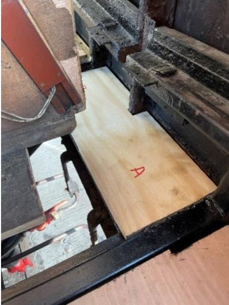
One of the compartments showing the repaired floor awaiting linoleum, and the overhauled reading lights being tested
