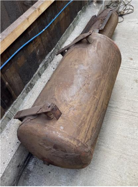
Old air reservoirs after removal – both subsequently failed testing due to corrosion
