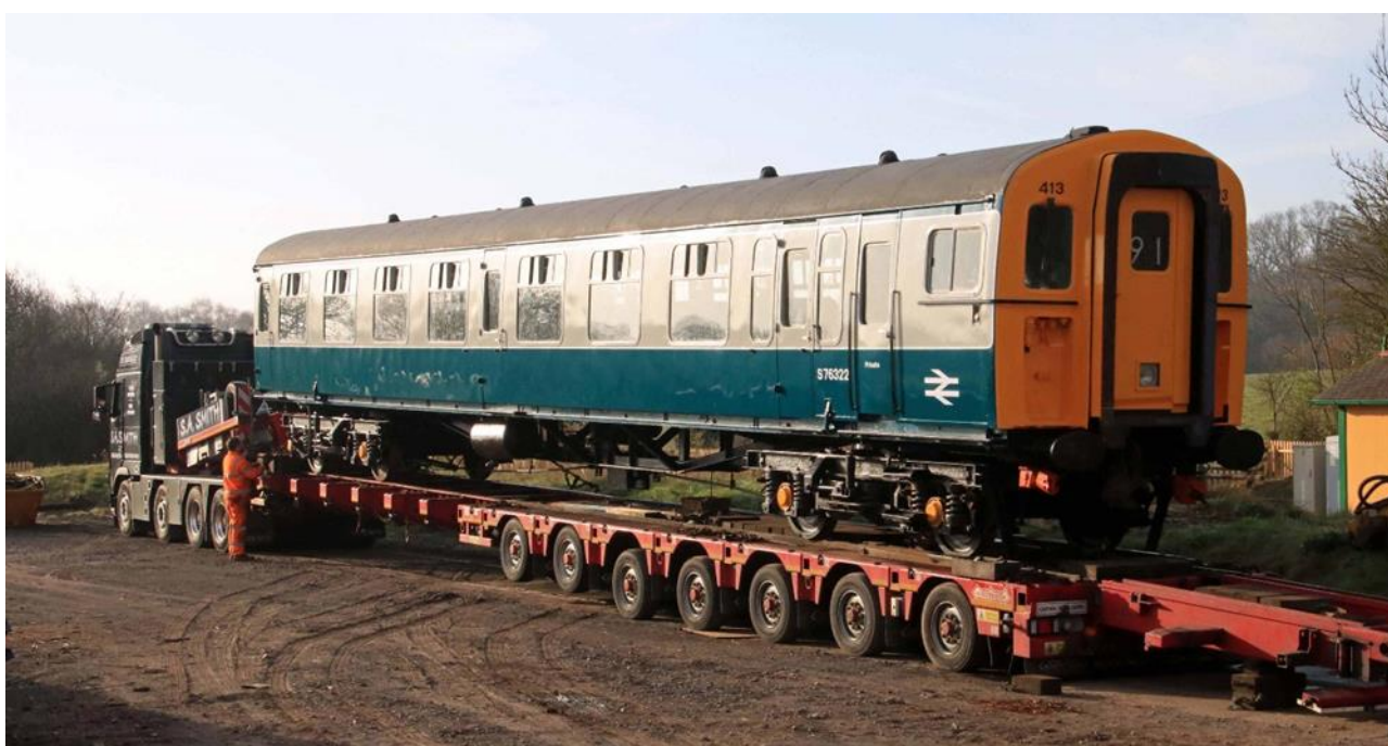
76322 being unloaded at Norden after bodywork restoration and bogie overhaul (30 th March 2021)
