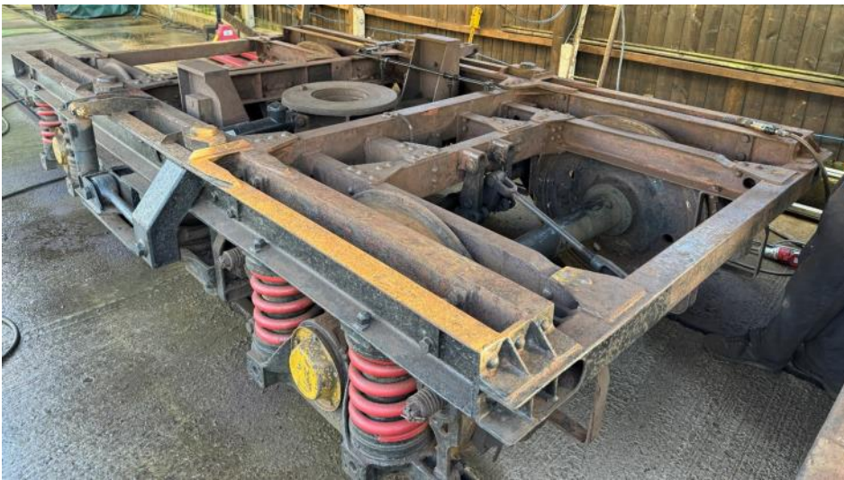
Bogie during needle gunning to remove old paint and rust.
