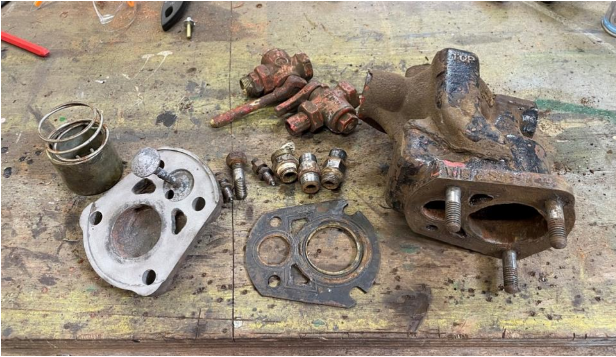
Air filter/strainer stripped for overhaul
