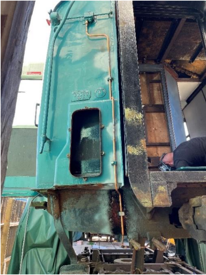
New brake pipework fitted to replace stolen sections
