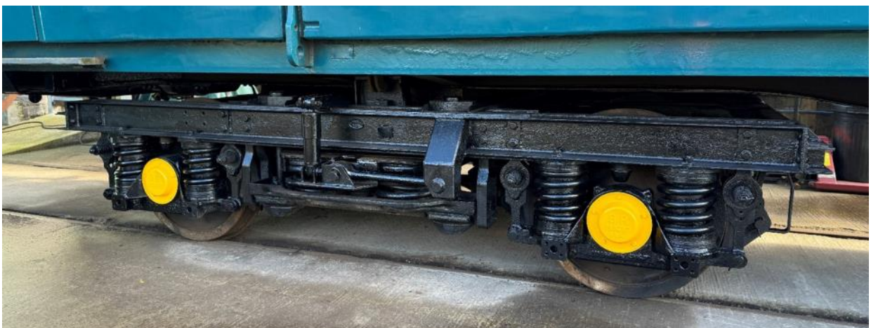
Bogie after spraying black with anti-corrosive paint, and yellow axlebox covers
