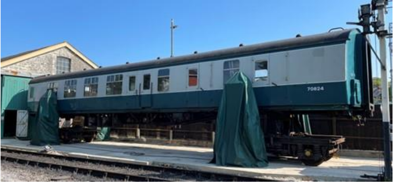
TBSK 70824 lifted off its bogies (13 th May 2023).
