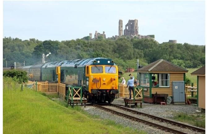
Here, the "Purbeck and Bomo Explorer" charter train, 12 coaches hauled by two heritage class 50 diesels, passes through Norden Gates level crossing under a clear signal, on its way back to Derby. Single line tokens are being exchanged by the conductor driver, Dave Gravell, and the crossing keeper, yours truly. ( I could have selected one of Andrew's pictures without me in it, but it wouldn't have been as good, would it?!)
