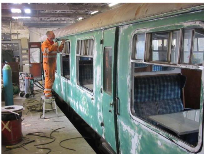
Inside, Jason Kingdon has removed the windows from BR Mark 1 2<sup>nd</sup> class open coach S4961, and is sealing the frames prior to applying a new coat of paint.
