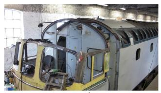
The cab at No. 2 end on 3<sup>rd</sup> June. Spot the new metal welded in. The fibreglass cab roof sections will also need some repair before re-fitting.
