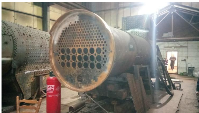
At the smokebox end of the boiler, a new front tubeplate has been fitted.
