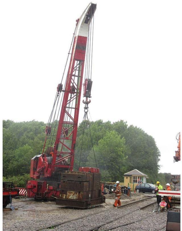
Here, Peter picks up the proof test load of weights borrowed from John Weaver. Steve checks the weight on his instrument connected to a load cell located in the rams horn crane hook. 57.8tonnes! That's 56.9 of your proper British tons.
