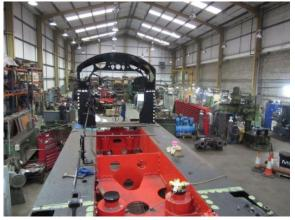
The rolling chassis, tender, and new smokebox of Battle of Britain class 34072 '257 Squadron', under overhaul by Southern Locomotives Ltd (SLL), are framed by the reconstructed cab of the 'N' class mogul.
