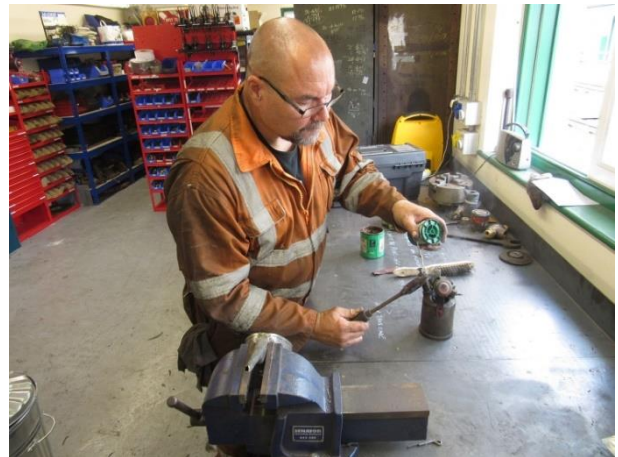
In the new workshop, diesel fitter Andy Garrett uses old technology to repair an oil feeder. Daisy the DMU says he's going to be busy this week!
